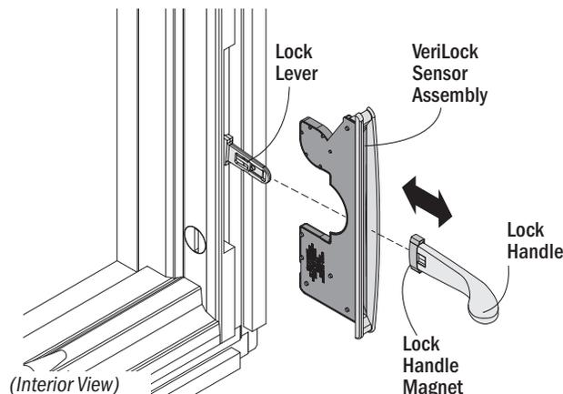
**NOTE:** VeriLock sensor assembly is installed on the **left** lock on awning units, as viewed from the interior.
